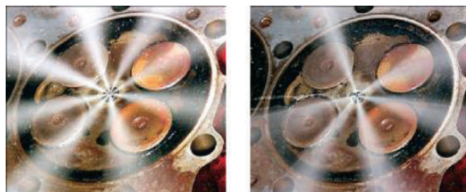
Close up of new (left) and worn (right) fuel injector nozzles.
